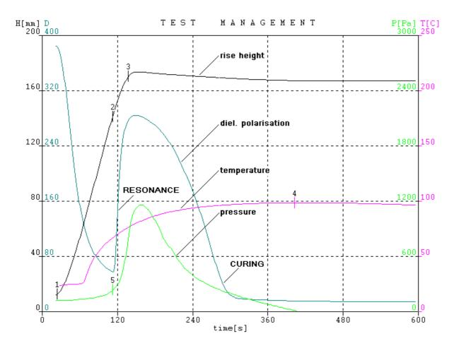
**Figure 2.** Dielectric polarization measured with CMD, and other physical data obtained for a molded foam. The polarization curve shows a significant resonance structure and the curing behavior.
