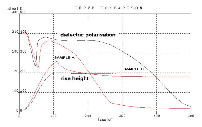
**Figure 2.** Comparison of the rise height and the dielectric polarization for two flexible foam samples with different isocyanate content. Sample B was made with 5/3 of the isocyanate amount of sample A.
