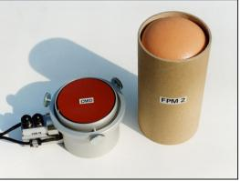
Fig. 4: The polarization sensor CMD, which is integrated into the FPM device measures the dielectric polarization of a foam sample patent 10104854 simultaneously with the rise pressure.
