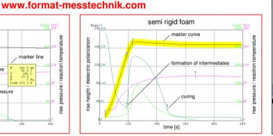
Fig. 3: Graphical display of the rise height, dielectric polarization, rise pressure, temperature, and master curve. The master curve is a tolerance band showing the margins of a "good" foam sample.
