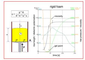
Fig. 5: The viscosity value is calculated by using the physical model of Hagen-Poisseuille, which is applied to a rigid foam measured with FOAMAT patent 19730891
