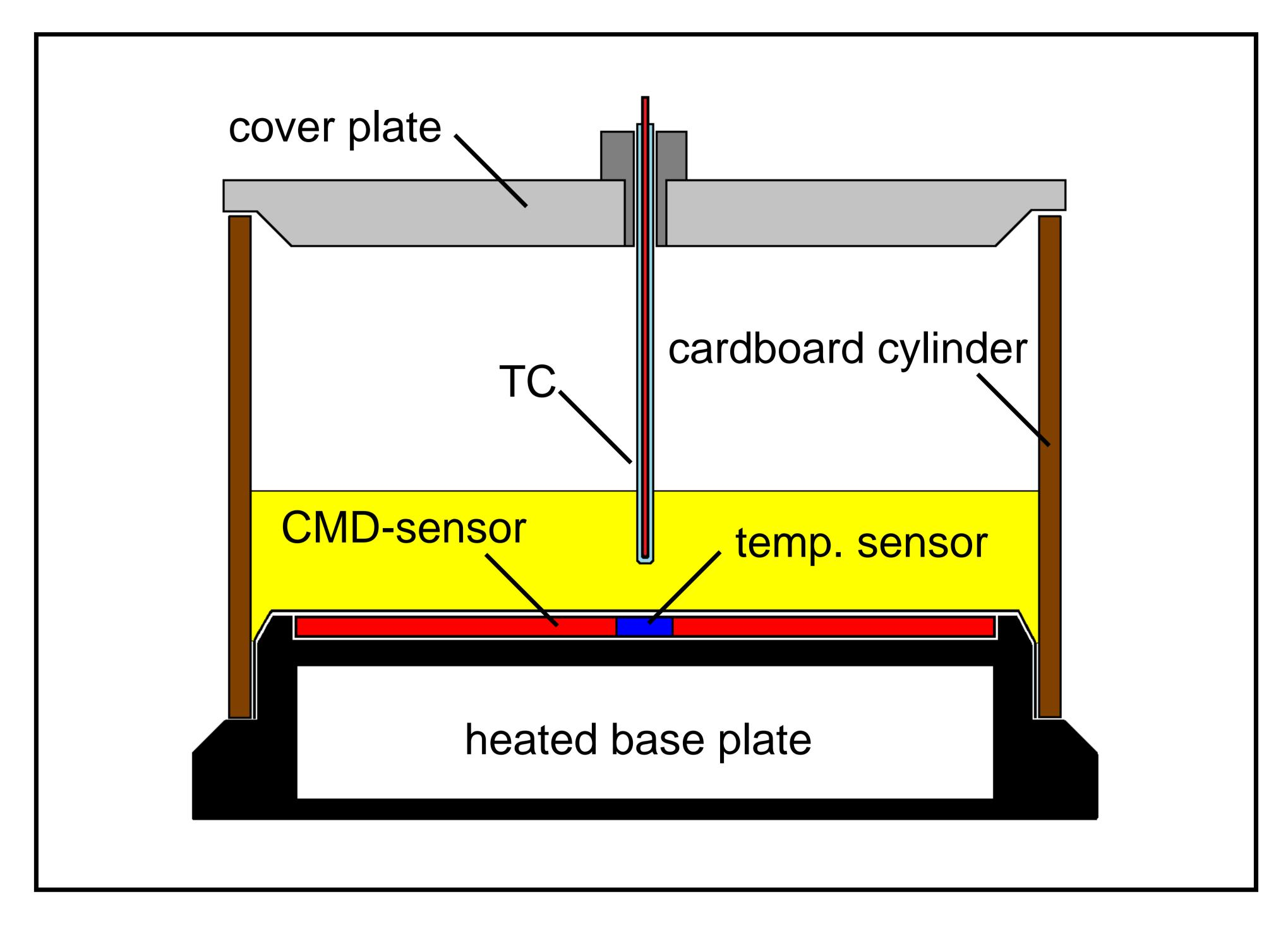
Fig. 5: Cross section of the SubCASE HT test container. The CMD-sensor is mounted onto the temperature controlled base plate. The core temperature is measured with a thermocouple.
