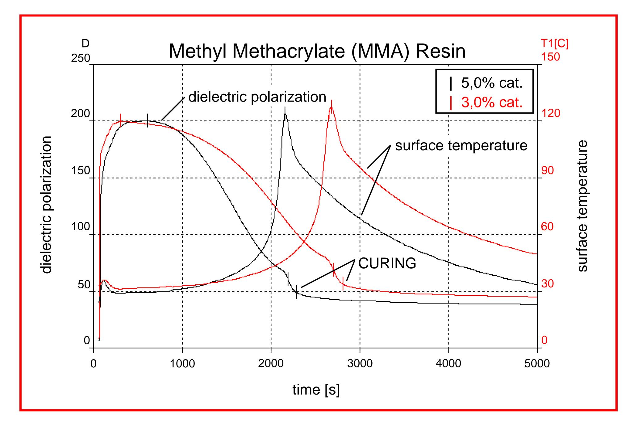
Fig. 4: Comparison of two methyl methacrylate (MMA) resins with different amount of catalyst. The different curing behavior is shown in the dielectric polarization curve D, as well as in the surface temperature curve T1.
