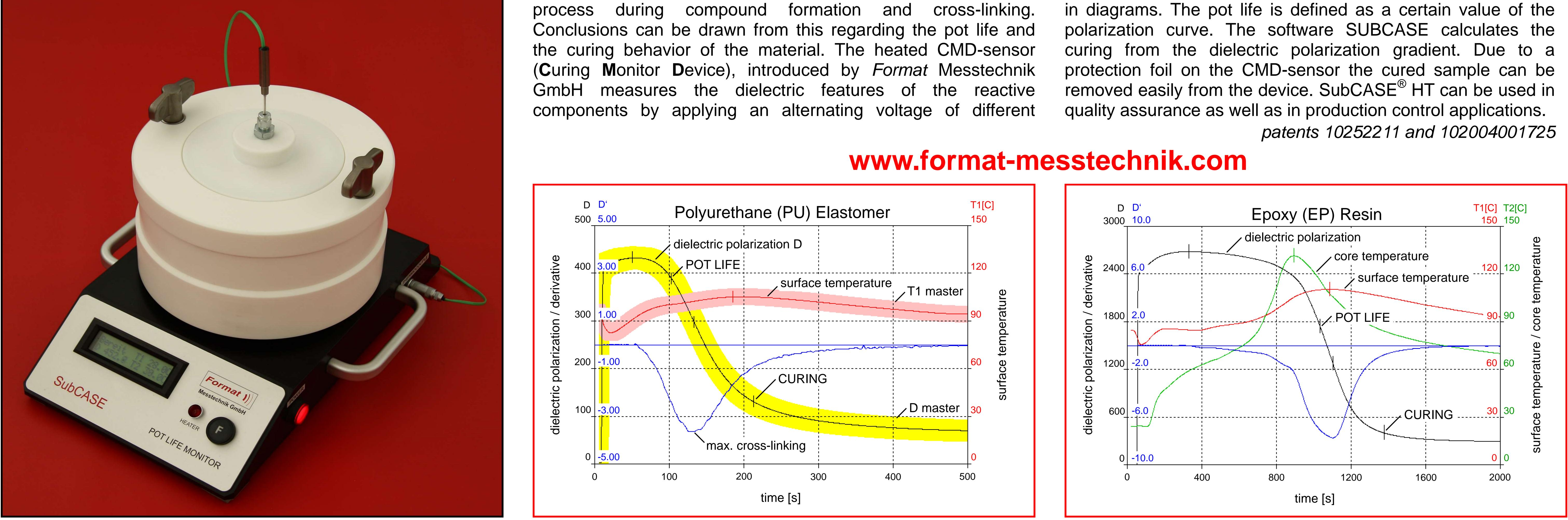
Fig. 1: Test device SubCASE HT for measuring the pot life and the curing of Coatings, Adhesives, Sealants and Elastomers (C.A.S.E.). The reaction profile is determined by dielectric polarization and temperature measurement.
