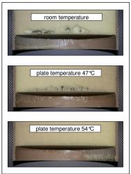
*Fig. 5:* Cross section of three samples of a flexible foam formulation, measured at three different bottom plate temperatures.
