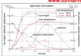
Fig. 2: Two sets of measurement curves of a rigid foam formulation, measured at different bottom temperatures of the test container. Depending on the temperature, the rise pressure and the dielectric polarization show most significant changes. polarization signals were affected most significantly by different surface temperatures (Fig. 2).
