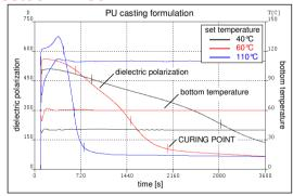
Fig. 3: Three SubCASE® measurements of a casting formulation measured at different bottom temperatures. The dielectric polarization shows strong temperature dependence: Curing goes faster with higher temperatures.
