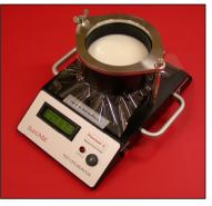
*Fig. 4:* The Pot Life and Curing Monitor Device SubCASE<sup>®</sup> and the high temperature test container filled with a white CASE formulation.
