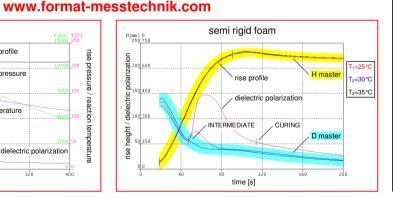
Fig. 3: The figure shows the variation of the dielectric polarization of a semi rigid formulation at three different temperatures. The H master and the D master are generated by the software FOAM for QC purposes.
