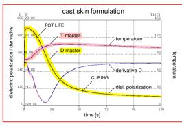
Fig. 5: Three dielectric polarization and temperature measurements of a transparent, fast curing cast skin formulation, which is used for fine wood decoration. The data show perfect reproducibility.
