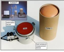
Fig. 1: The polarization sensor CMD2, integrated into the foam pressure measurement device FPM2, measures the dielectric polarization of the foam in combination with rise profile and temperature.
